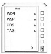
This is the wind mode prompt screen used when solving for heading/groundspeed. In this case, wind direction (WDR) and wind speed (WSP) plus course (CRS) and true airspeed (TAS) are required. Use the scratch pad to enter the variables in the following sample problem. It is a must that you state your entire wind problem in true or magnetic and stay with the same reference throughout each problem.
