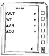
First enter gross weight (GWT) and weight (WT) in the respective parameter lines. In these problems, the delta sign (\*) means a change in values. In this problem, the required change in center of gravity (\*CG) is -5 inches. In other words, the CG must move forward 5 inches for the aircraft to be within limits. When you enter 5 inches in the \*CG parameter line, \*AR is lined out. This means that \*AR will be the value solved for when you press compute.
