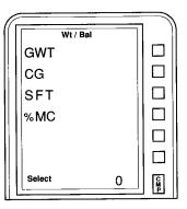
Notice the Wt/Bal mode prompt is illuminated at the top of the screen and select is showing at the bottom. The menu select screen allows you to select the type of problems you wish to solve. In the weight and balance mode, you have three choices for prompted solutions:
