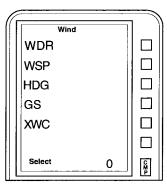
Notice wind is illuminated at the top of the screen and select is showing at the bottom. The menu select screen allows you to select the type of problems you wish to solve. In the wind mode, you have three choices for prompted solutions:
